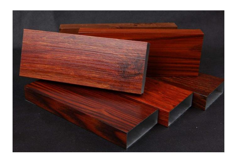
woodgrain like aluminium extrusion Simulation of wood, extruded aluminum first spraying primer, and then the grain on the surface of pasted paper, through vacuum heating process, the penetration to wood completely uniform to the spraying primer.
